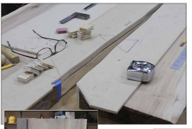
Joe Scannell built a desk from an elm he harvested in Nicasio in 2013. The primary wood for all the parts came from that tree. The desk top is made from two 2" thick slabs that he joined in such a way that part of the desk is 21" deep (plus a retractable keyboard extension), and the remainder is 30" deep.
