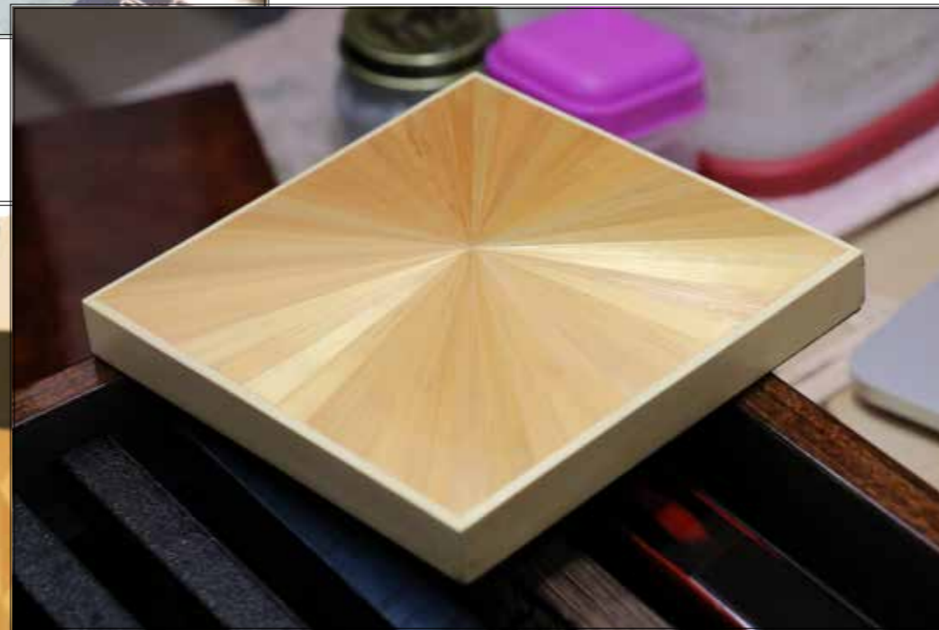
Renowned wood finisher Joe Amaral also came over from Fort Bragg, not selling anything, just there to share his knowledge. We discussed lacquer and, of course, his amazing use of straw, which he imports from France, splits and flattens with an iron, and uses as veneer, as seen above.
