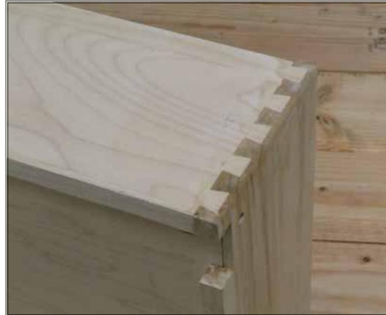
its way into the inside of the drawer, making a mess that is difficult to clean up. His solution is to spray some accelerator on the inside of the drawer before applying the CA; any glue leaking through will go off before it can become a problem.
