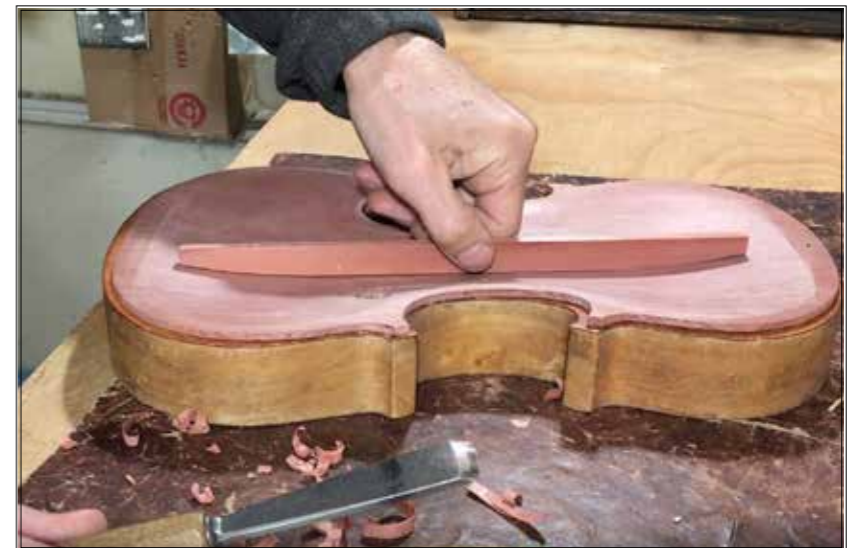
Fitting the redwood bass bar to the front
